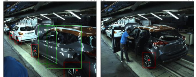
Figure 15 Left: Successful left front wheel detection; Right: Failed left front wheel detection.
